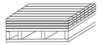
Green Atlantic PVC trim, sheet and Moulding products should be stored on a flat and level surface. PVC products are more flexible than wood, they may deform on uneven surfaces. Ensure that storage areas, as well as all framing and substructures, are flat and level to minimize uneven surfaces.
